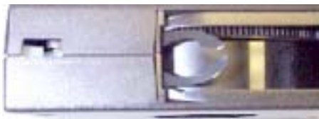
Figure 1-26. Media wrapped too loosely (improper tension)
